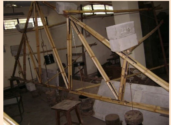
(b) Bamboo truss (Sonar and Siddhaye, 2009)
