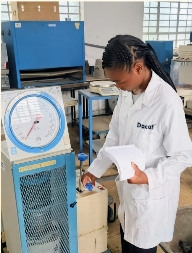
A student using the Compression Testing Machine (CTM) at the Materials lab
