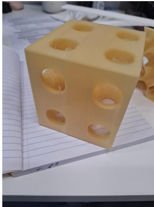
Figure 2: 3D-printed mold used for fabricating nacre-like structures in concrete The concrete specimens, after casting, are then cured and kept for 28 days at specific temperature and humidity conditions. This process also ensures that the full strength of each concrete sandwich is realized, as well as the bond between the layers and the tubular inclusions.
