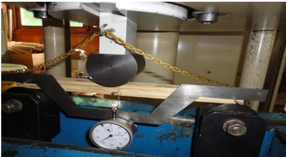
Figure 3.6: Static bending test setup dimensions
