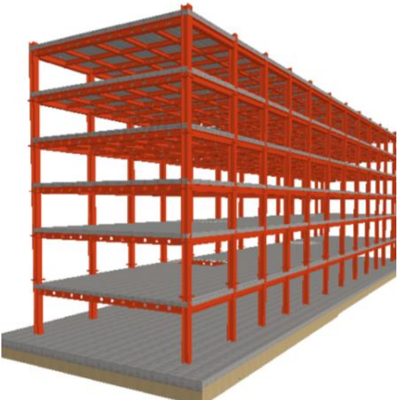
Step 5: Fixing of decking sheetsStep 6: Fixing of upper floor columns and pouring of concrete on ground floor
