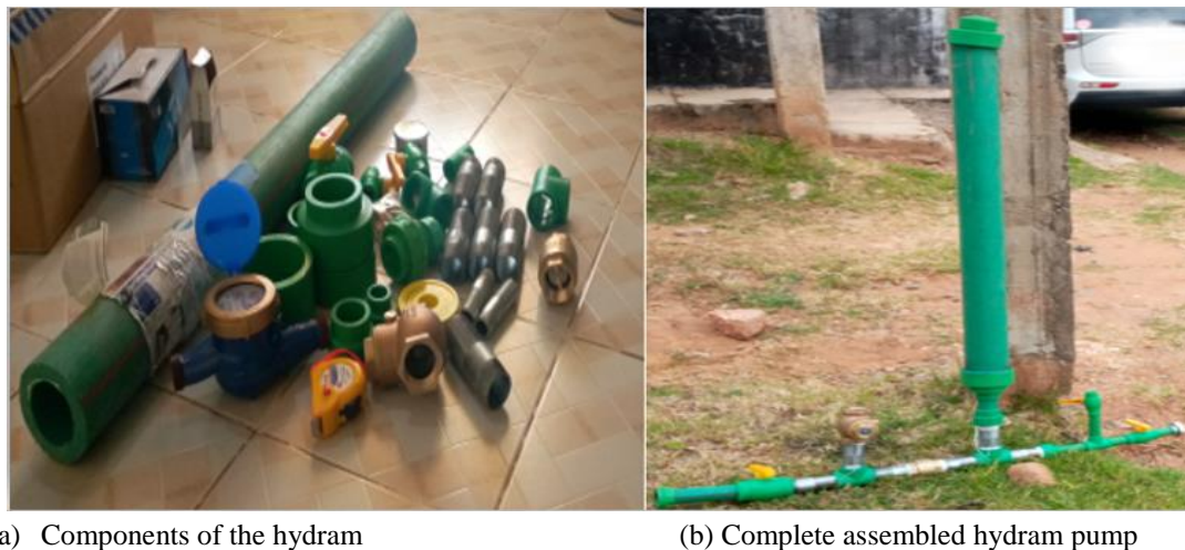
Figure 4: Fabrication of the Hydam pump (Source: Actual Site Photographs).
