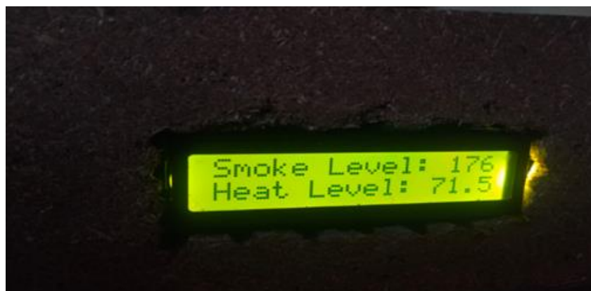
Figure 8: LCD Display after fire detection.
