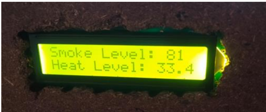
Figure 7: LCD display of smoke and temperature before fire detection.
